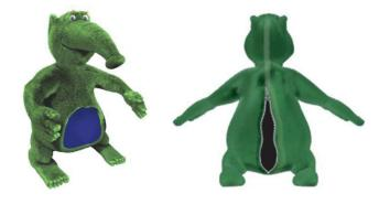
Figure 2: Computerized 3D representation of Probo, with removable fur jacket.
